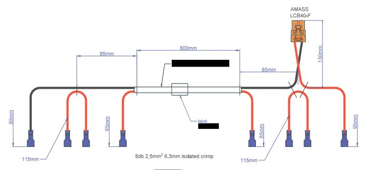
article: wire: red and black as in the draw 2,5mm², FLRYW or silicon isolation, or similar what is like the shake. For AMASS connector need extra fill in wire.
